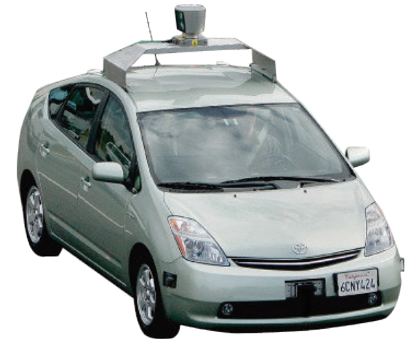
Google's modified Toyota Prius uses an array of sensors to navigate public roads without a human driver. Photograph by Ramin Rahimian
