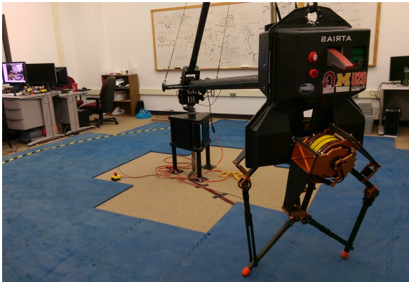
Figure 6.17: 2D experimental testbed of ATRIAS. The left picture shows the actual testbed of ATRIAS constrained to a circular track by a boom (A). We use a high-fidelity simulation of this testbed to investigate virtual neuromuscular control (B).
