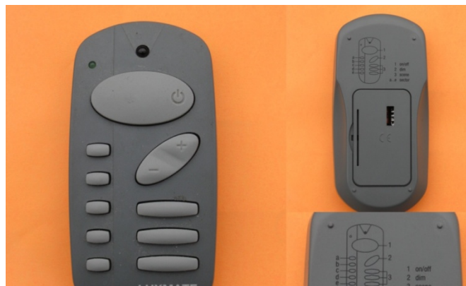
Figure 2.2.1 LUXMATE remote lighting controller
