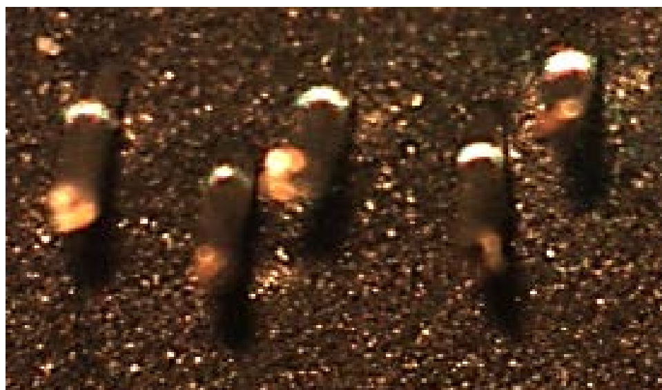
5-12: OCT MARS v2 with 5 pin calibration phantom. The top surfaces of the pins are highlighted by the overlay.
