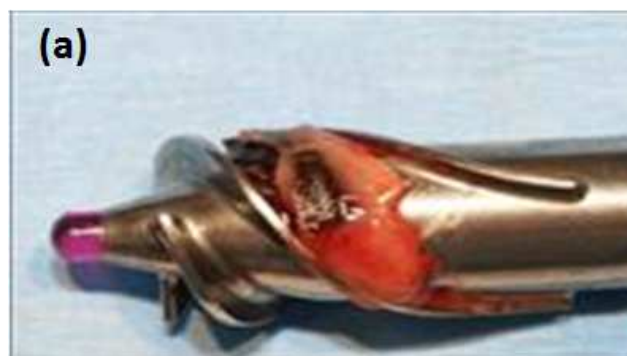
Figure 4.13 Thrombus deposition procedure in axial blood pump: the straightener vane and the impeller. The inlet flow rate is 2.0L/min. The rotational speed of impeller is 9000RPM.
