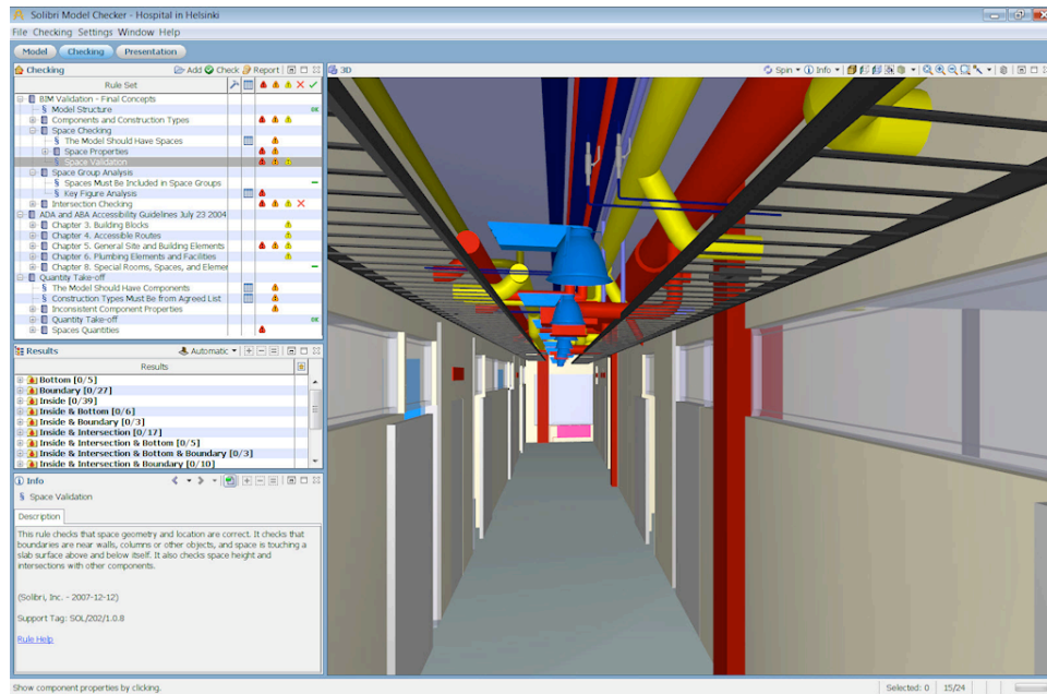
Figure 2.8 Solibri Model Checker: when a user selects an item (in this case, space ventilation) in the left window, the system presents its review, and then the system highlights relevant parts in the 3D model.
