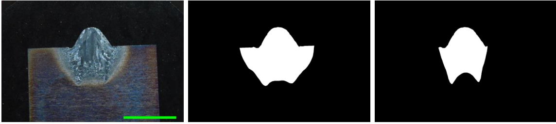
Figure 98. Sample 2-8. Experiment line 2, eighth section in transient region.
