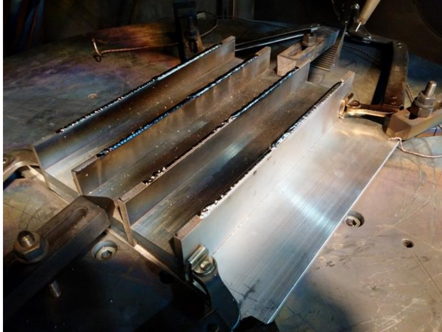
Figure 43. Example thin wall experiments post deposition.
