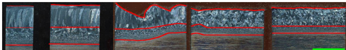
Figure 88. Example cross section to view melt pool depth (Experiment 1, Transient Section).
