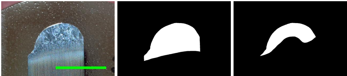
Figure 45. Polished cross-section (left) and the measurement of the heat affected zone (middle) and melted portion of the wall (right) for the initial steady state of experiment line 1. Green scale bar is 0.25 in.
