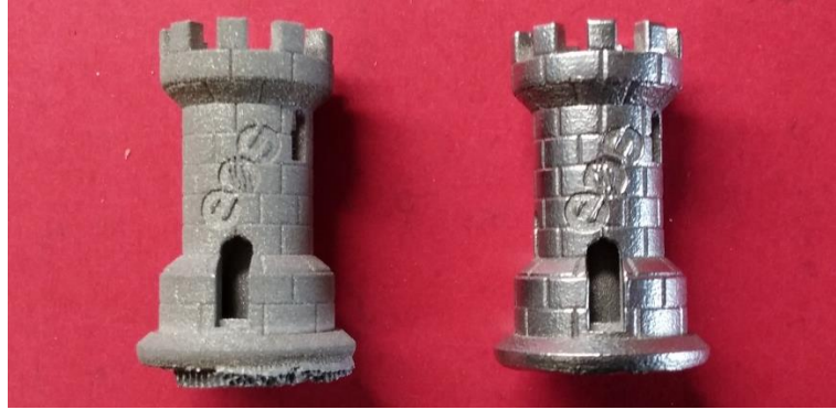
Figure 2. An example of a part built through AM prior to removing excess material (left) and after removing excess material (right).
