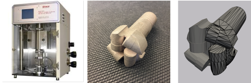
Figure 11.1: Benchtop drilling simulator (left), miniaturized drill bit (center), stl file of the drill bit to be used in simulations (right)
