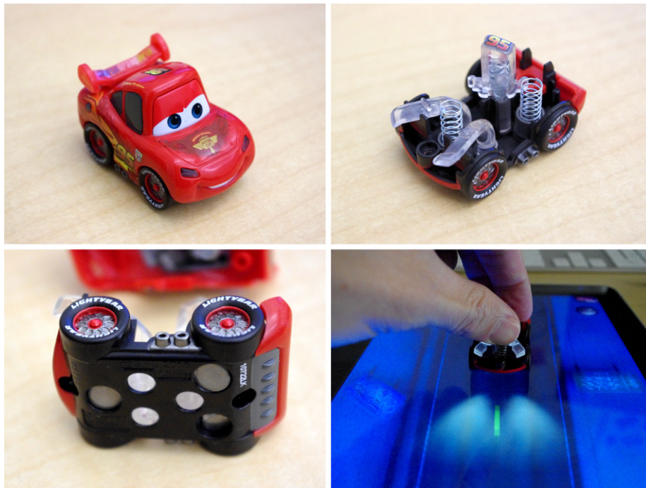
Figure 79: A commercial car toy with embedded light guides that direct light from a tablet computer into the headlights.
