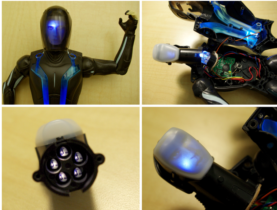
Figure 78: A commercial figurine with a simple LED projection mechanism to create an animated face.
