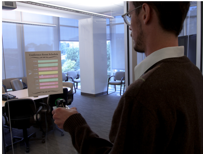
Figure 70: The Schedule Viewer application enables a static sign to be augmented with projected information from a conference room schedule.
