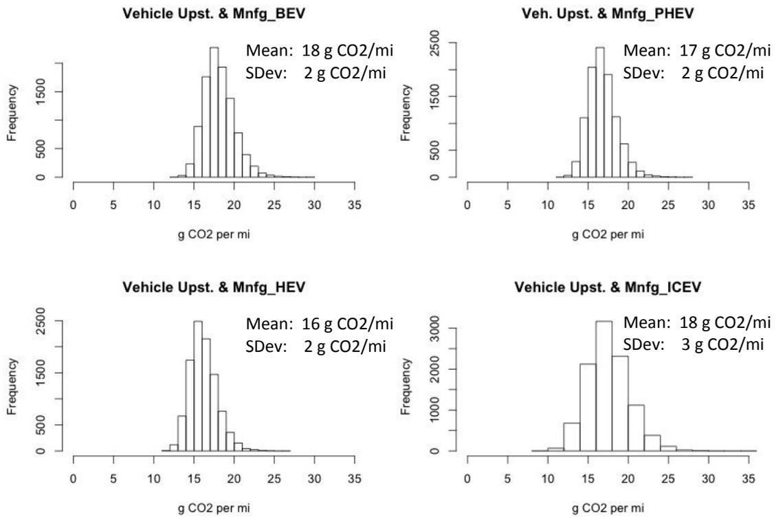
Figure 26. Vehicle upstream and manufacturing emissions estimates by vehicle type - Battery electric vehicle (BEV), Plug-in hybrid electric vehicle (PHEV), Hybrid electric vehicle (HEV), and Internal combustion engine vehicle (ICEV).
