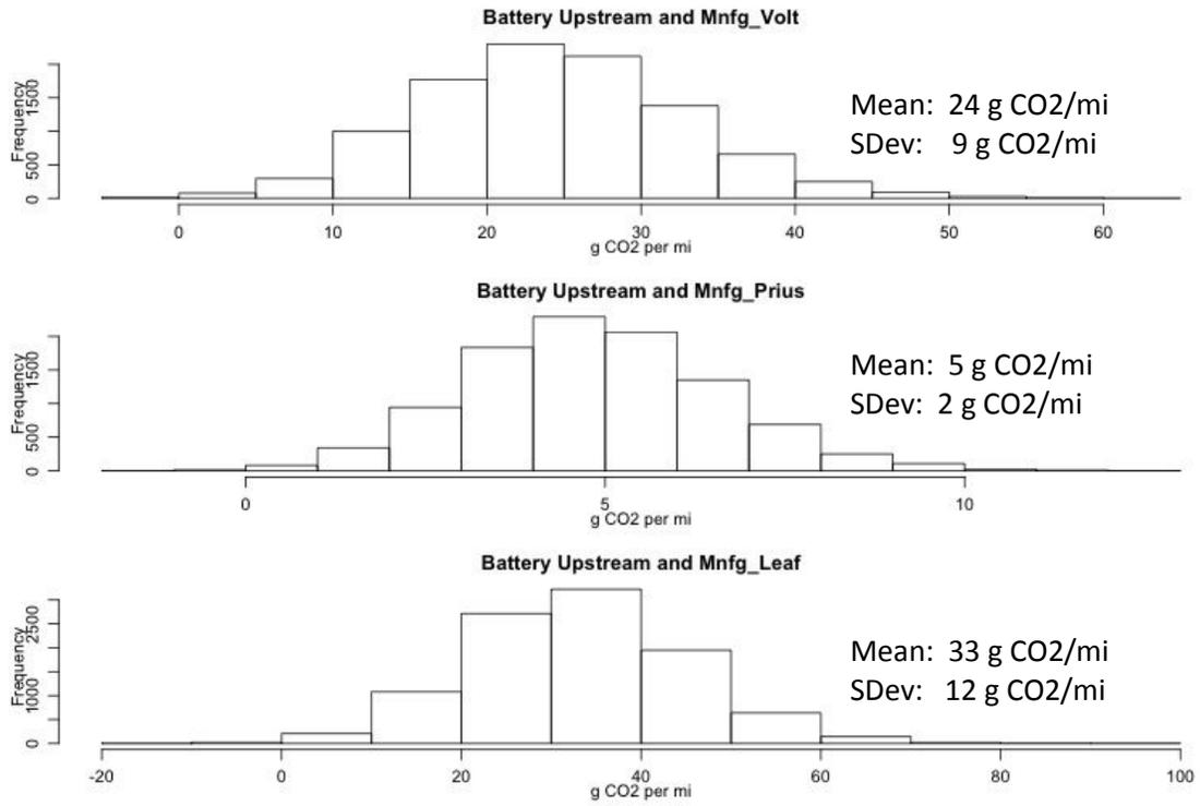
Figure 25. Lithium-ion Battery upstream and manufacturing emissions estimate for Chevrolet Volt, Toyota Prius PHEV, and Nissan Leaf
