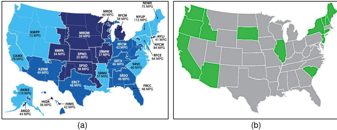
Figure 9. (a) EV Ratings comparing Nissan Leaf to gasoline vehicle using 2009 eGRID subregion avg. emission factors [Violet = EV is comparable to gasoline vehicle with 31-40 mpg); Blue = EV is comparable to gasoline vehicles with 41-50 mpg; and Light Blue = EV is comparable to gasoline vehicles with >51 mpg)] (Anair & Mahmassani (2012)); (b) Leaf vs Toyota Prius HEV using 2010 State Average Emissions Factor (Green: Leaf is lower emitting), Source: Yawitz, et al. (2013))
