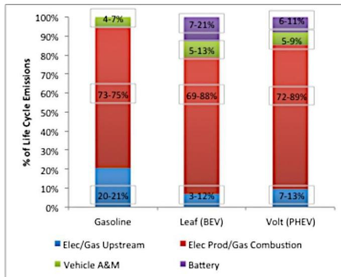
Figure 14. Life cycle emissions by vehicle type using marginal emission factors for Evs.
