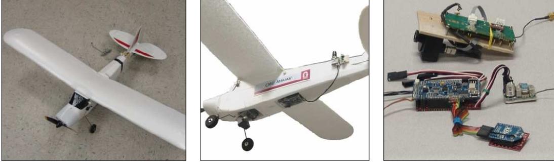
Figure 6.2: UAV testbed platform and onboard components
