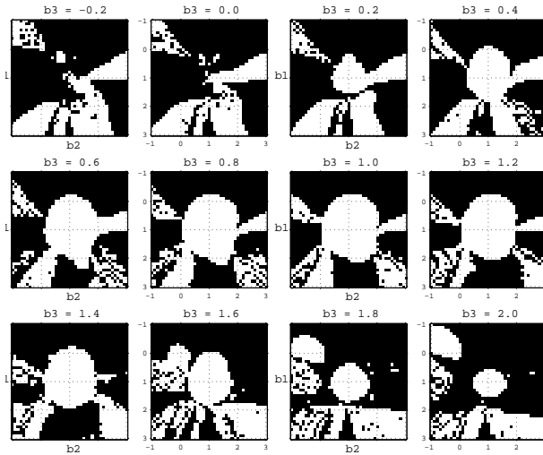
Figure 4.8: Bias convergence region of the iterative factorization for a triad-IMU. Each plot is a cross section along b_3 . Initial conditions, \mathbf{b}^0 = [b_1 \ b_2 \ b_3] , in the white region converge to the true \mathbf{b}^* = [1 \ 1 \ 1] but those in a non-white region are trapped in local minima.
