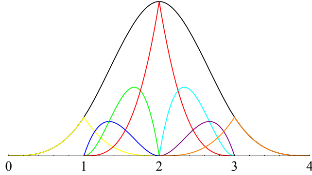
Figure 5.17: T-spline basis function N(\xi) (the black curve) defined on the knot vector \{0, 1, 2, 3, 4\} and the extracted seven weighted Bézier basis functions (curves rendered with different colors). The seven weighted Bézier basis functions are defined on \{0, 1, 1, 1, 2\} , \{1, 1, 1, 2, 2\} , \{1, 1, 2, 2, 2\} , \{1, 2, 2, 2, 3\} , \{2, 2, 2, 3, 3\} , \{2, 2, 3, 3, 3\} and \{2, 3, 3, 3, 4\} , and the weights are 1/6, 1/3, 2/3, 2/3, 2/3, 1/3 and 1/6 , respectively.
