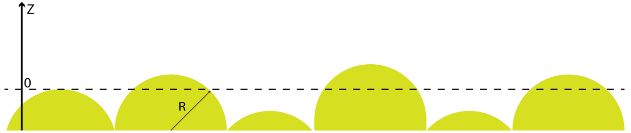
Figure 2.4: Schematic of the Greenwood-Williamson model assumptions. Surface roughness asperities are assumed as spherical asperities with the same radius with different height distributions.
