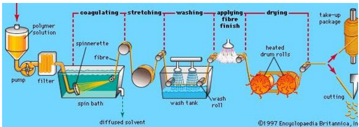
Figure 2.3: A Wet spinning process in which polymer solution or gel is extruded through a spinneret and solidified in a coagulating bath. Image from Britannica Inc.
