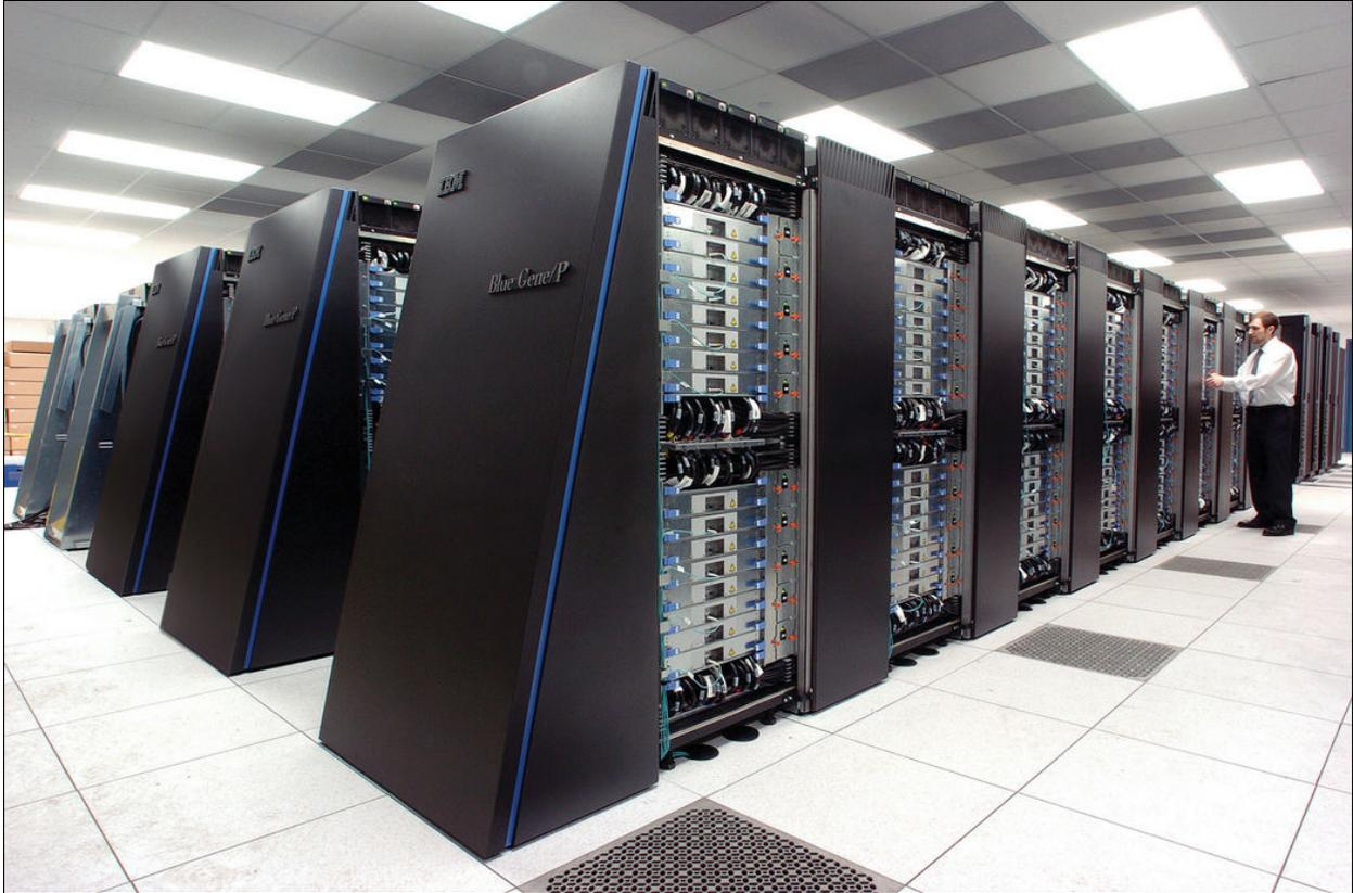
Figure 1.1: Intrepid, consists of 40 Blue Gene/P racks [3].
