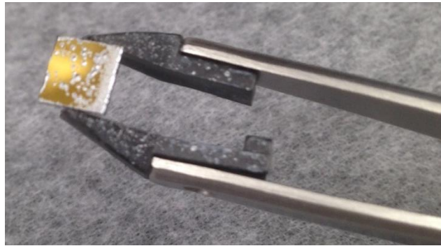
Figure 5.48: Backside view of the gyroscope after it is demounted from the DIP40.
