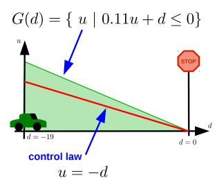
Figure 3.4: Illustration of refinement: control envelope contains control law
