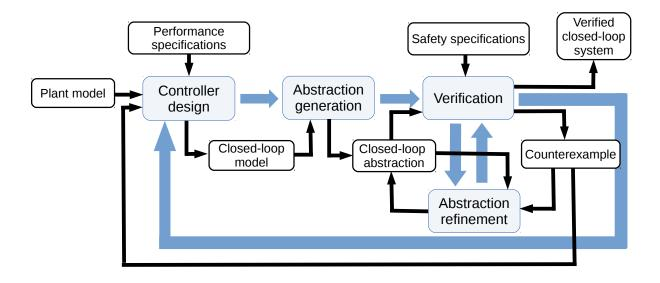
Figure 3.1: Conventional approach: design according to performance specifications, abstract the closed-loop system and apply formal method to verify safety.
