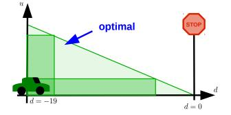
Figure 3.5: The parametric envelopes are underapproximations of the optimal control envelope
