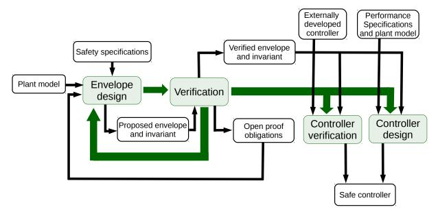
Figure 3.2: Proposed approach: design control envelope according to safety specifications. Proceed to controller design or verification after the control envelope is verified.
