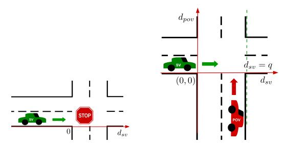
(a) Stop sign assist stage 1, SV approaches inter- (b) Stop sign assist stage 2, SV must traverse insectiontersection while avoiding POV
