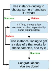
Figure 4.1: Procedure for parametric refinement checking
