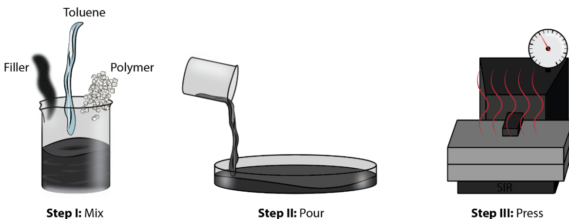
Figure 3.1: Procedure for the preparation of conductive PCL sheets. Step I: PCL pellets are added to a mixture of carbon filler and toluene, and stirred until the mixture becomes homogeneous. Step II: The mixture is poured into a large petri dish and the solvent is allowed to evaporate. Step III: The resulting conductive PCL is compressed with a heat press to create a flat homogeneous sheet.
