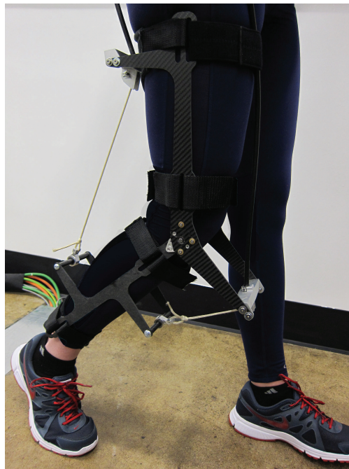
Figure 2.9: Knee exoskeleton featuring a simple pivot joint and plate carbon fiber frame.
