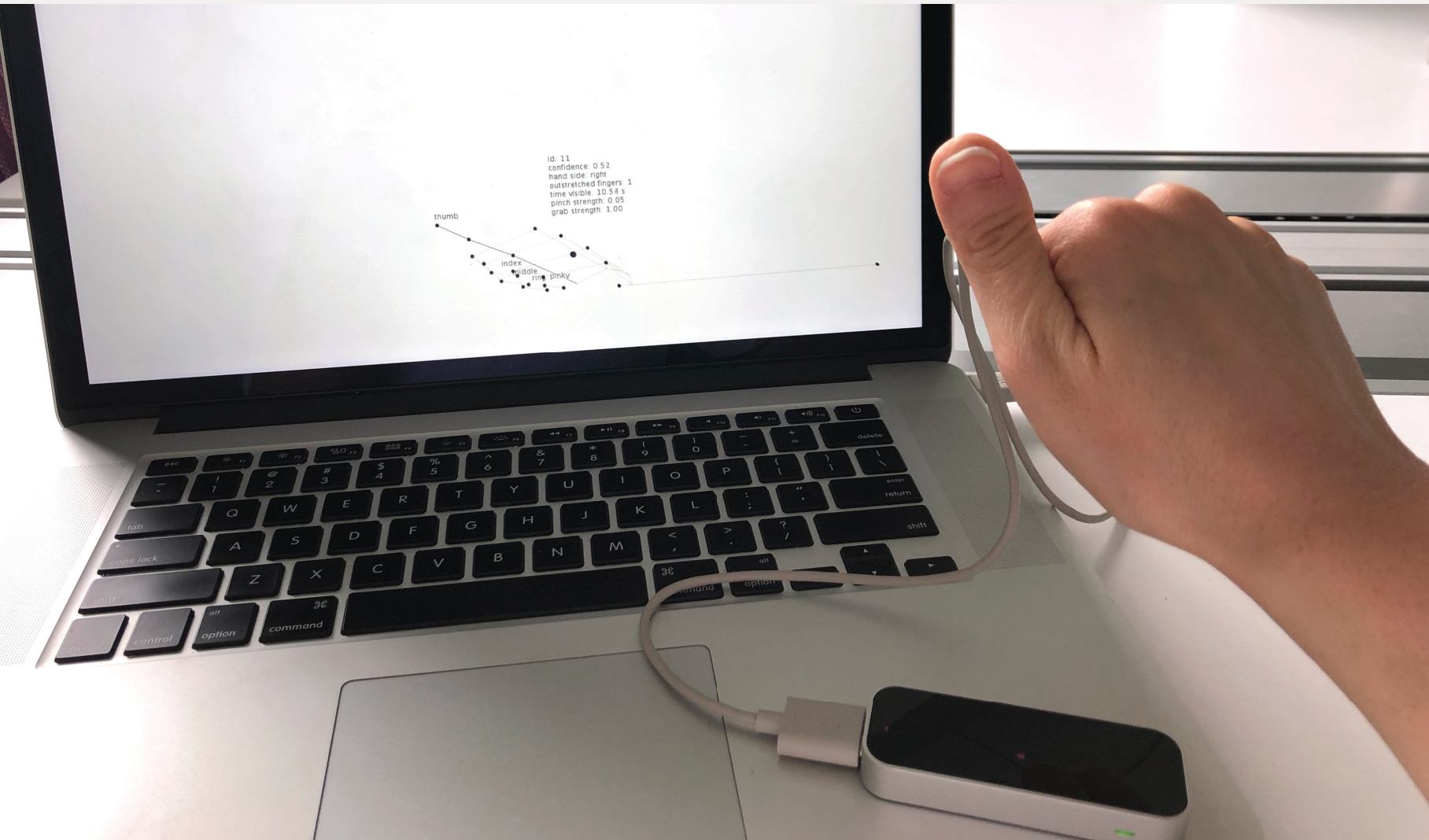
Figure 23 Processing visualizing hand and finger data via Leap Motion
