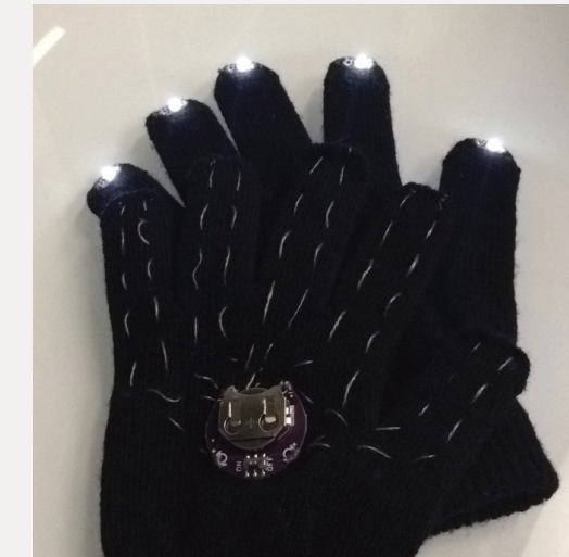
Figures 11 & 12 Light gloves made to use with long exposure photography in order to capture the participant signing.
