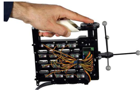
Figure 24: TextureTouch, reprinted from “ NormalTouch and TextureTouch: High-Fidelity 3D Haptic Shape Rendering on Handheld Virtual Reality Controllers ” 76
