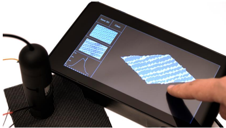
Figure 46: Interface and Visualization of 3D Texture Scanner System Prototype
