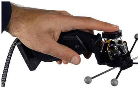
Figure 23: NormalTouch, reprinted from “ NormalTouch and TextureTouch: High-Fidelity 3D Haptic Shape Rendering on Handheld Virtual Reality Controllers ” 75
