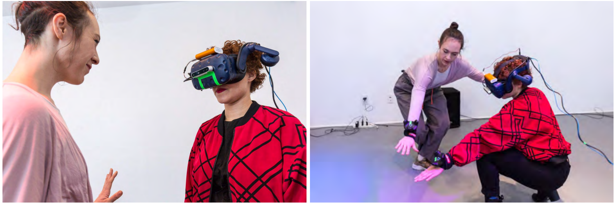
Figures: Participant interacts with dancer, wearing HTC Vive Pro with Intel RealSense camera mounted on the front, allowing a real time streamed depth video of the dancer to be seen.
