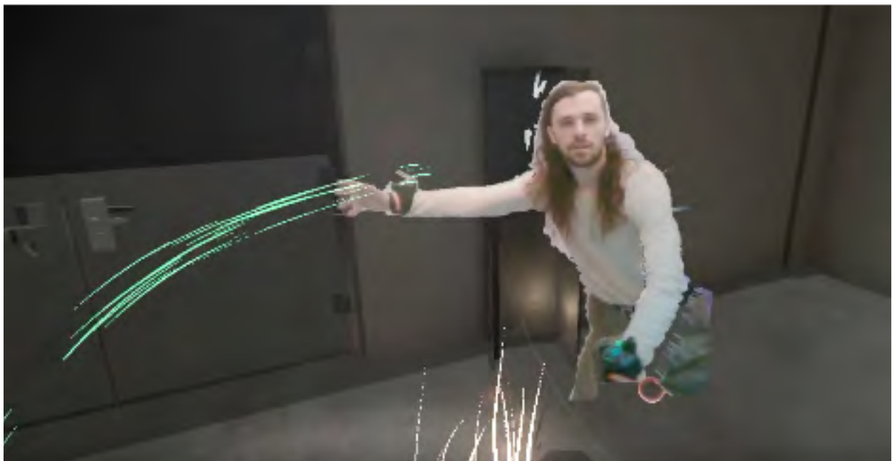
Figure: In-headset view of co-located, co-present dancer (Taylor Knight) streamed through Intel RealSense camera. Dancer and participant can interact with shared virtual objects which participant sees in-headset, and dancer sees on external monitor in the physical room.
