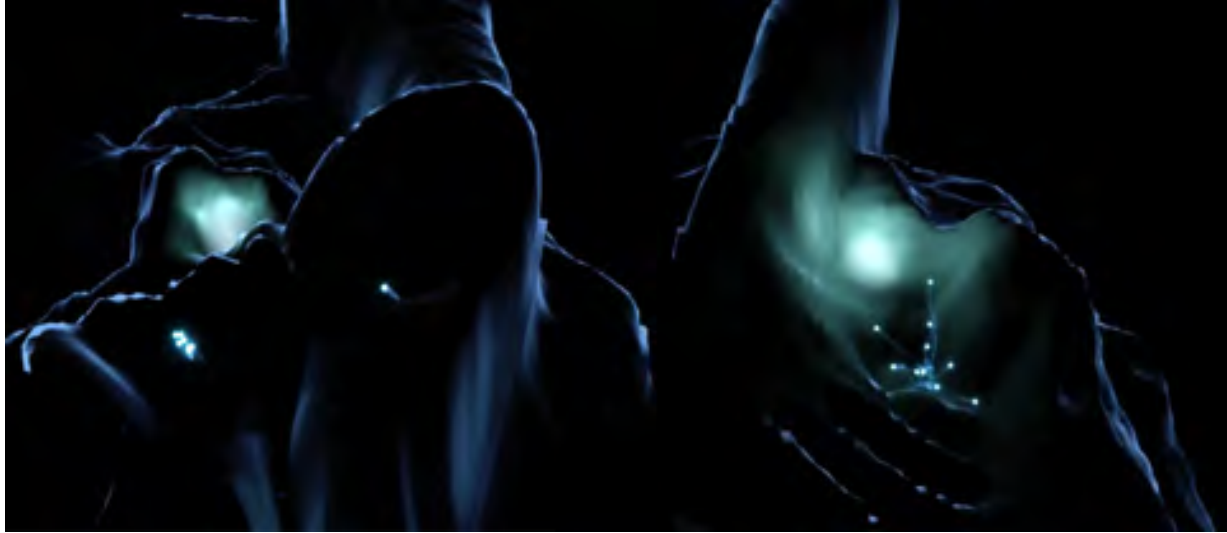
Figure 7. Views in player headsets, using Oculus Touch. Depth mesh rendered with rim light shader, virtual spheres visible, and virtual light triggered by player touch.
