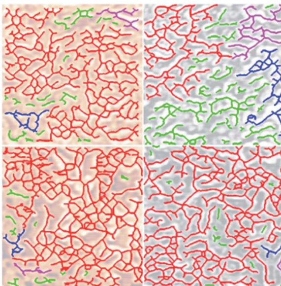
Figure 4.4 AFM images of BCP film (left column) and resultant CTNC-700 (right column) for two extreme catalyst loadings: 12 \mu\text{g}/\text{cm}^2 (top row) and 180 \mu\text{g}/\text{cm}^2 (bottom row).
