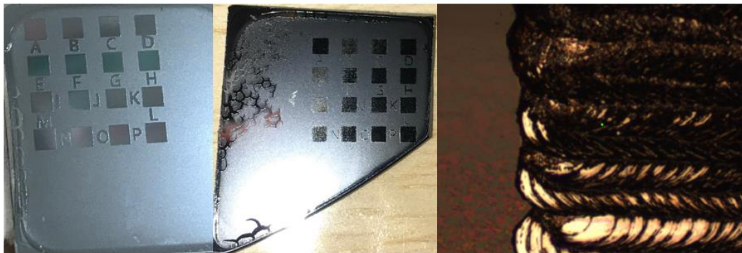
Figure 3.4 Drop cast PAN- b -PBA films on silicon exposed to CO 2 laser radiation of differing speeds and powers, both without any prior stabilization of the film (left) and with oxidative stabilization (middle). (Right) Optical microscopy image (10× objective) of a stabilized PAN- b -PBA film on silicon. Stabilized PAN- b -PBA that was not exposed to the laser is on the left and laser exposed is on the right with visible effects from lines from the CO 2 laser's rastering.
