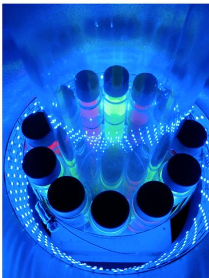
Figure 1-13. Side illuminating photoreactor design developed by the Bernhard group. Reprinted with permission from ref<sup>41</sup>. Copyright American Chemical Society 2013.
