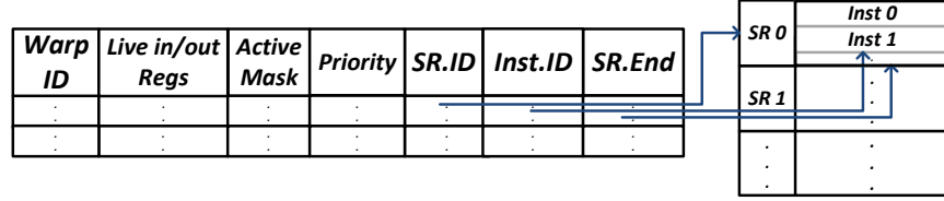
Figure 47: Fetch Logic: Assist Warp Table (contained in the AWC) and the Assist Warp Store (AWS).
