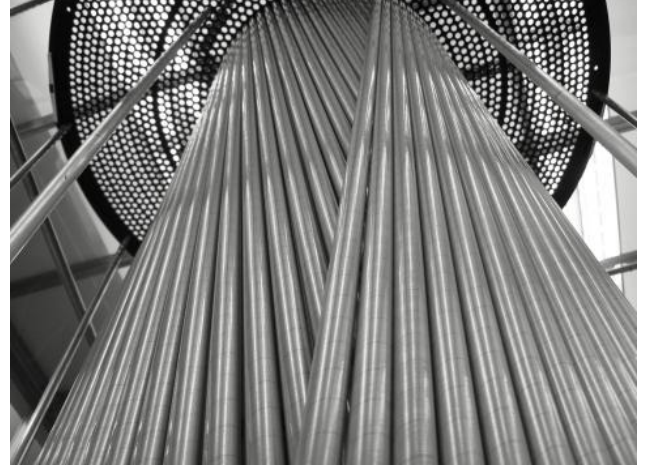
(b) Picture showing parts of layer of opposite-direction stereo straws before the rest of the straws were strung [61].
