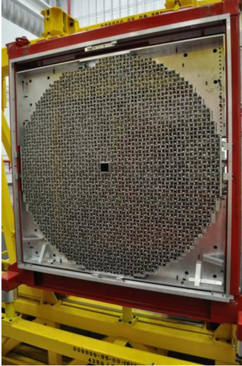
Figure 2.20: View of the front face of the FCAL before the dark room enclosure has been installed behind it [61].
