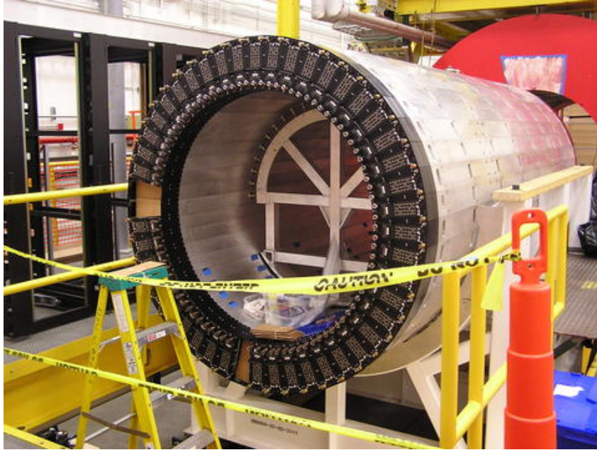
Figure 2.24: View of the upstream face of the BCAL before being inserted into the solenoid bore [76].
