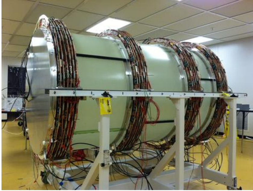
Figure 2.16: View of the FDC before being inserted into the solenoid magnet bore. The 4 FDC packages are visible as the thick bands of readout cables [61].
