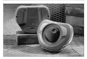
**Figure 7.16** Evolution of a wearable computer through various iterations of prototypes: a) form prototypes; b) breadboard prototypes; and c) final VuMan 3 developed at Carnegie Mellon University. (Reprinted with permission of Dan Siewiorek, Ivo Stivoric, and Chris Kasabach)
