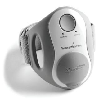
Figure 1.7 Original SenseWear System from BodyMedia. (© Image courtesy of BodyMedia, Inc.)
