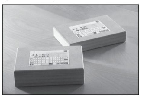
**Figure 5.4** Block-level prototypes that are precursors to a hand-held augmentative communications device. (Reprinted with permission of Daedalus)
