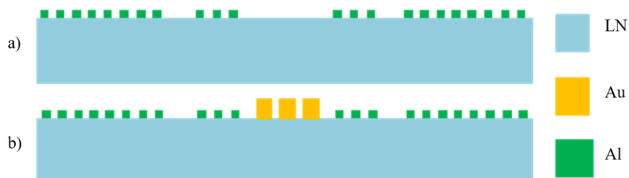
Figure 3.1: Fabrication process flow for making the SAWG. a) Al lift-off step used to define the electrodes.
