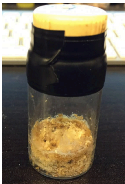
Figure 63. Lithium/mPEG composite prepared without the addition of LiTFSI. V(\text{Li})/V(\text{PEO})=1/3 . The sampled showed low homogeneity and a solid-like form.
