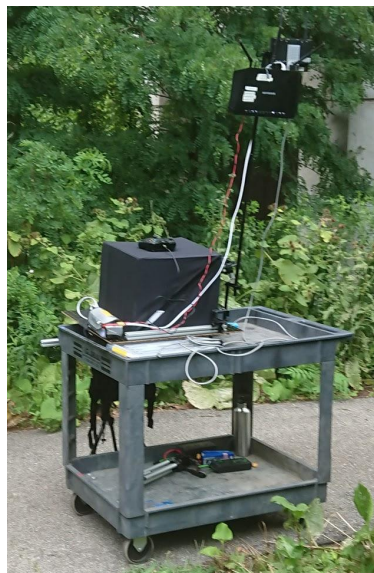
Figure G.6: Cart-mounted ground control station. The router is on a vertical boom to improve wifi range. A black IKEA DRONA storage box shields the base station laptop from direct sunlight.
