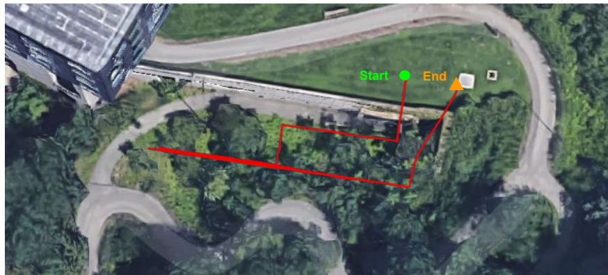
Figure 3.11: Estimated flight path over treetops superimposed on satellite imagery
