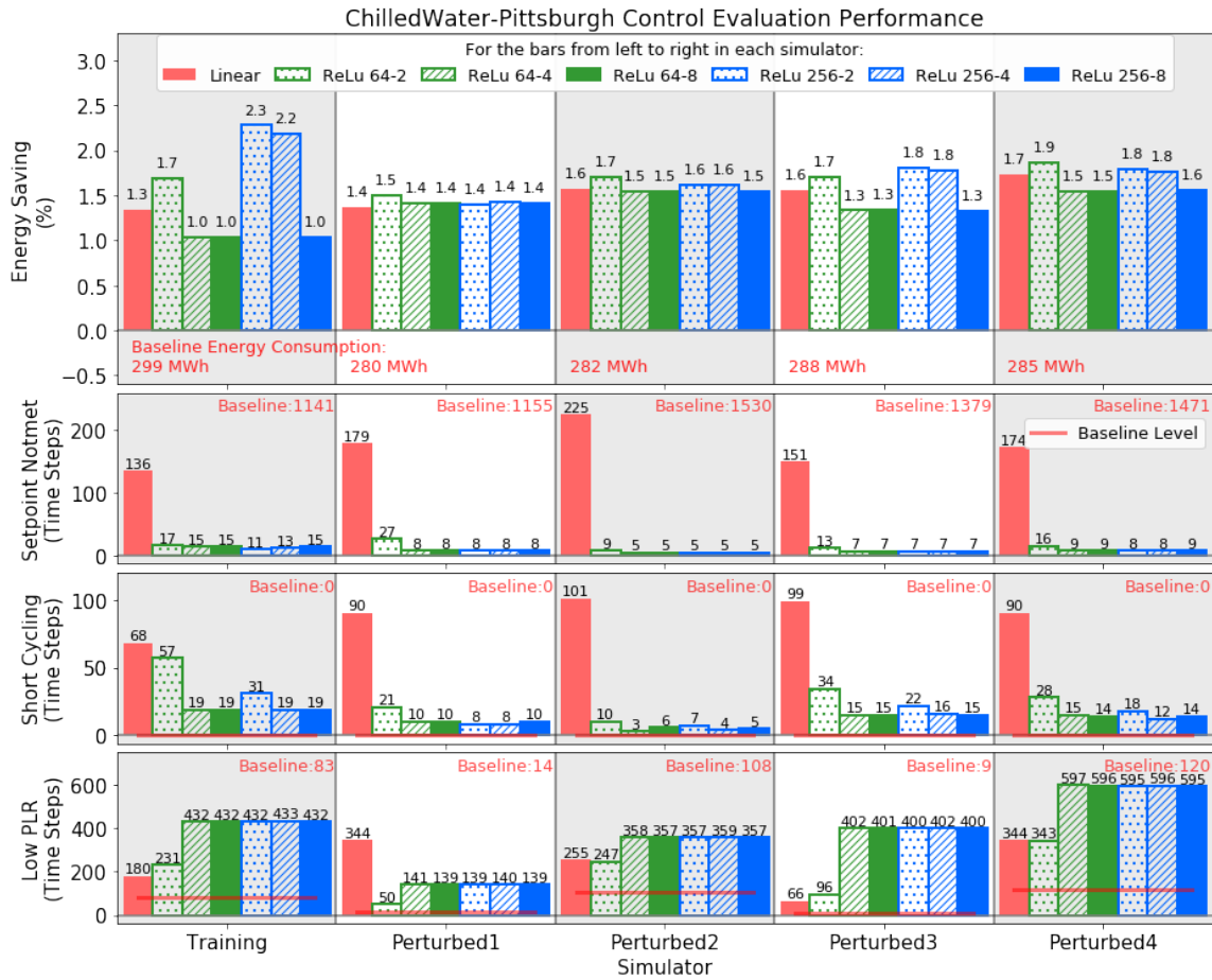
Figure 7.11: ChilledWater: Control Performance in Pittsburgh Climate (the results of each neural network model are from the best-performing learning rate)
