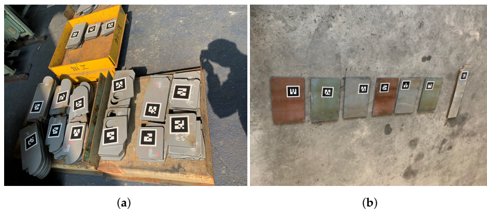
Figure 3. Workpieces tagged with AR markers used for experiments at the shipyard. (a) Real-world workpieces within the shipyard viewed by a worker. (b) Test environment where the workpieces were moved by workers to evaluate our system under real-world mover behavior.
