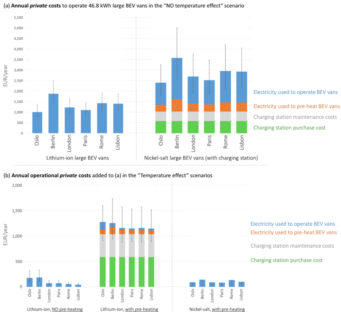
Fig. 3-6 46.8 kWh large BEV van operational (a) and additional (b) private costs due to temperature effect. Uncertainty bars are mainly due to driving conditions, annual mileage and electricity prices and refer to the whole columns. For comparison, diesel van costs are in the order of 6,500 to 12,000 EUR/year, depending on the city.
