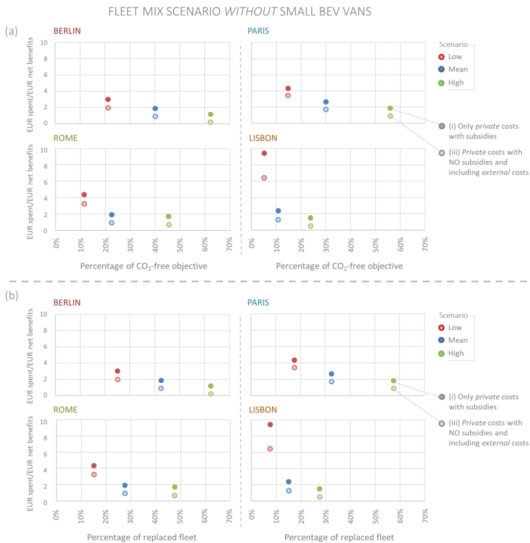
Fig. 5-23 Relative comparison across cities' low-carbon vehicle fleets without BEV vans, in terms of “ private costs per external cost savings ” and “ percentage of mileage or fleet replacement ” in the cities of this study. Estimates assume riders are paid the minimum wage and the replaced small diesel vans have 0.4 average load factor.
