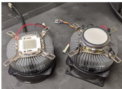
Figure 4.5 LED assemblies allow for easy modification of the Lightbox 2.0 to experimental needs. On left, a bare LED unit, on right, an LED unit directed through a frosted dispersing lens to improve illumination uniformity across larger samples.
