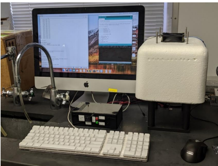
Figure 4.4 Lightbox 2.0 assembly with all elements visible (computer, illumination chamber, control box and light shield; left) and only illumination chamber without light shield (right).
