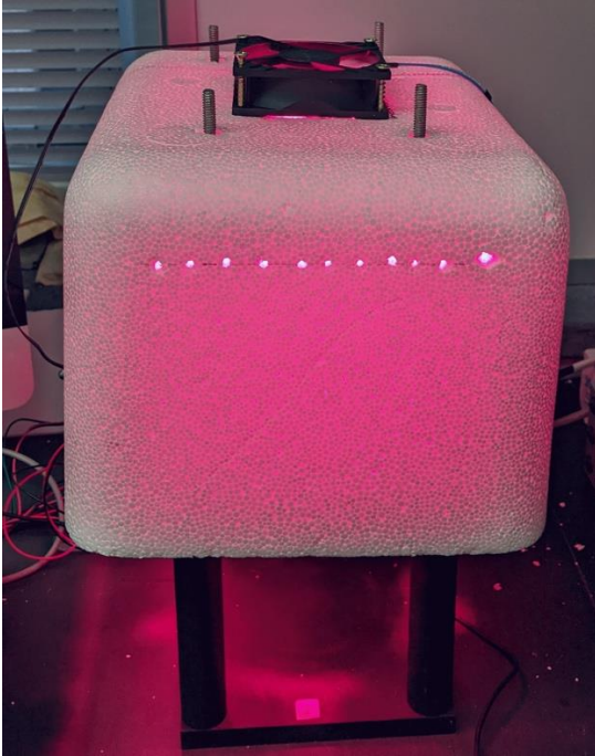
Figure 4.9 Light bleed through the Styrofoam light shield (left) and lightbox modifications to increase light reflections (right)
