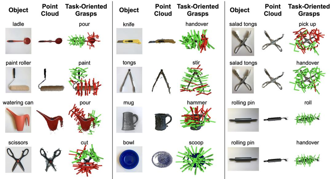
**Figure 7.1:** Example point clouds and grasps from our TaskGrasp dataset. Column 7-9 shows how grasps vary with tasks for a salad tongs (with higher diversity) and a rolling pin (with lower diversity). Green and Red means successful and incorrect task-oriented grasps respectively.
