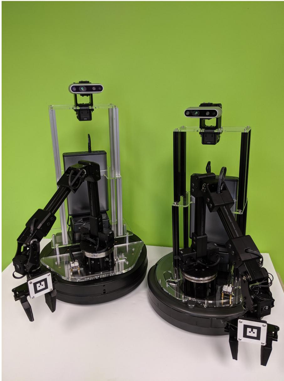
**Figure 5.2:** LoCoBot (left) and LoCoBot-Lite (right). Both robots have a 5 DOF arm mounted on top of a mobile base (Kobuki or Create2). Robots are equipped with a RGB-D camera mounted on a pan-tilt stand. Robots come with a battery pack and an on-board computer.
