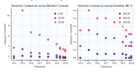
Figure 10 Dielectric constant as a function of frequency. A (left) varying moisture content %. B (right) varying density (unit kg/m³)
