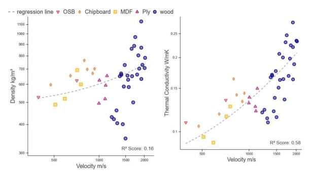
Figure 52 Scatter plot of sound speed vs density:
