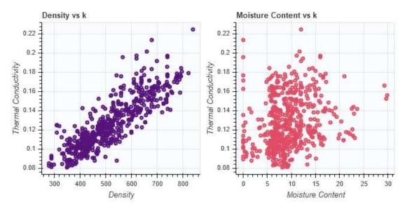
Figure 8 A (left) Scatter plot between thermal conductivity and density. B (right) Scatter plot between moisture content and thermal conductivity
