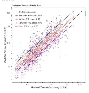
A. Comparison of various equations to predict thermal conductivity through moisture content and density.
