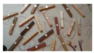
Figure 27 Prepared samples for the sound impact method (sound speed)
