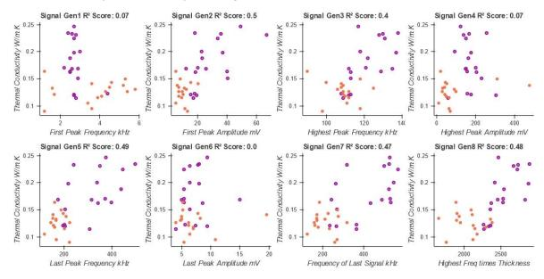
Figure 54 Results from signal gen: Thermal conductivity vs sound properties
