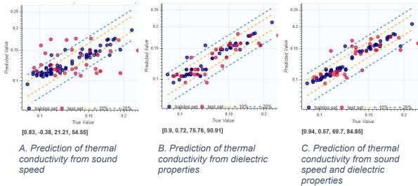
Figure 12 Predictions of thermal conductivity from Dielectric and Mechanical properties
