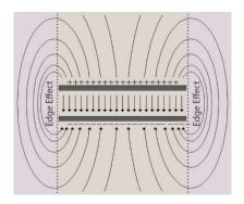
Figure 40 Edge effect between two plates of a capacitor is shown in pink
