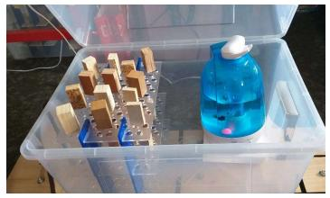
Figure 31 Humidity box containing humidifier, samples and humidity sensor.
