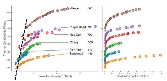
Figure 67 Thermal conductivity as a function of dielectric constant for all the woods measured for study 1. Size indicates moisture levels
