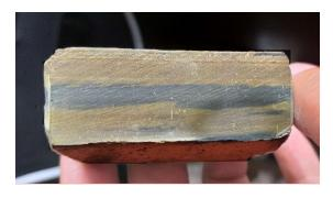
Figure 89 The Taxila stone is anisotropic and has veins of variable thickness running through it
