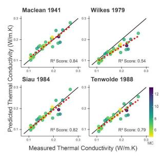
Figure 47 Comparison of measured data with predicted data from equations 5 to 9. The color of the dots indicates the moisture content, black line represents the line of perfect agreement, and dotted line represents regression line of data as per suggestion of scientist equation.
