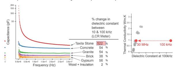
Figure 90 Frequency Sweeps with NanoVNA. Numbers to the right represent average % change in dielectric constant between 10 kHz and 100 kHz as measured by LCR meter
