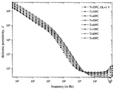
Figure 71 Change in dielectric constant of water with increased frequency below 10 megahertz as shown by Rusiniak [124]
