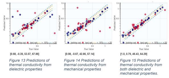
The numbers in the parenthesis indicate [training score, test score, % readings within 10% accuracy, % readings within 20% accuracy]
