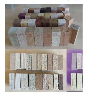
Figure 45 Material samples for solid wood (above) and wood-based materials (below)
