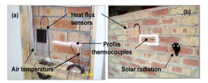
Figure 1 (Left) Sensors embedded in walls during the study by Luo et al [25]. Some of the sensors were painted the same color as the wall in an attempt to match the absorbance and emissivity of the walls.
