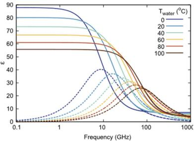
Figure 72 Change in dielectric constant of water at room temperature with increased frequency in gigahertz range as shown by Andryieuski et al [125]
