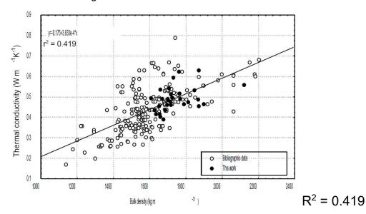
Figure 97 Correlation of bulk density and thermal conductivity of clay bricks as shown by Dondi et al [136]
