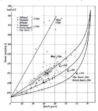
Figure 6 Thermal conductivity vs specific gravity for wood and woodbased panels reproduced from Siau [14]
