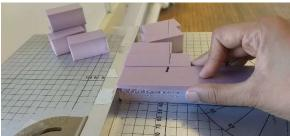
Figure 21 Foam Cutter (foam insulation)
