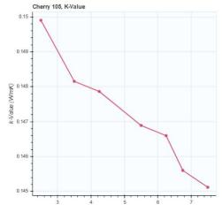
Figure 39 Readings of thermal conductivity for wood sample No 105.
