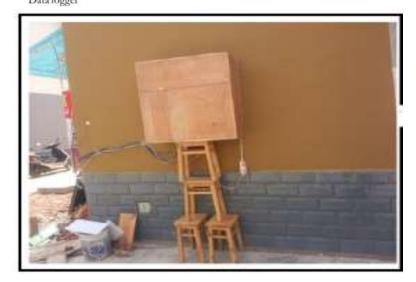
Figure 4 Hot box as described by Meng et al [31]
