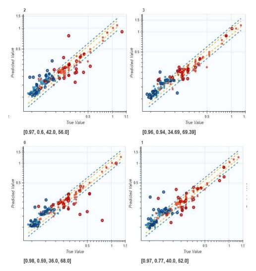
Figure 16 Four-fold cross validation results from wood and plastic combined. Red dots relate to wood, and the blue dots relate to the plastics data. The small squares represent training data, while the larger round symbols represent the test data
