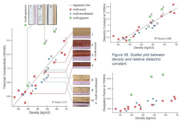
Figure 59. Scatter plot for density and thermal conductivity. Variation in insulation thickness affects both density and thermal conductivity.
