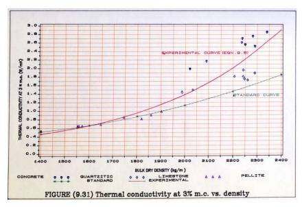
Figure 95 Ganjian's work on thermal conductivity of concrete and its density
