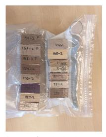
Figure 30 Samples inside vacuum bags meant to retain oven dry condition of samples
