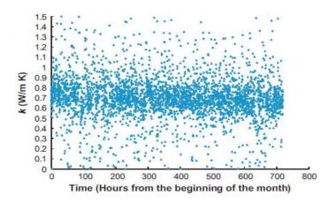
Figure 2 (Left) One data point of measured thermal conductivity for every ten minutes as per the study by Luo et al. Measured values seem to swing between 0 and 1.5 in every 24-hour period
