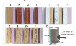
Figure 57 Samples 1-4: Hardwood-insulation. 5-7: gypsum drywall with insulation or solid wood. 8-11 OSB samples, first without air, then with layer of air. 12: Typical sample with dimensions.
