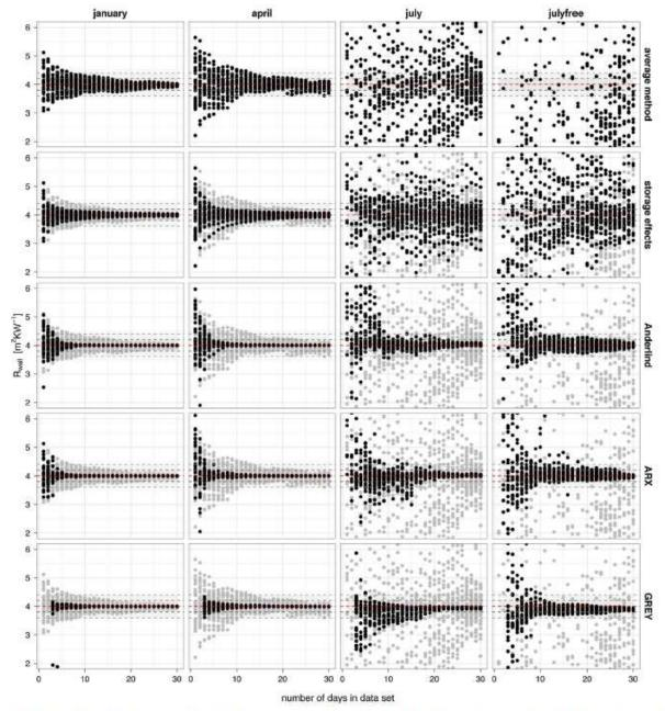
Fig. 3. Comparison of the different analysis techniques regarding the data set length and period. The red dotted line represents the reference value for the thermal resistance of the cavity wall. The grey dotted lines and areas correspond to the 5% and 10% accuracy bands. (For interpretation of the references to color in this figure legend, the reader is referred to the web version of the article.)
