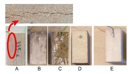
Figure 73 Adverse effects of the moisture content on the samples.
