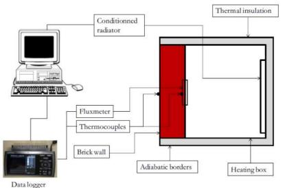
Figure 3 Configuration of a Hot-Box as described by Sassine [30]
