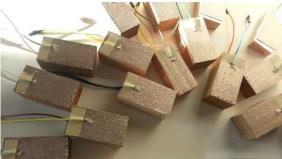
Figure 26 Prepared samples for dielectric measurements
