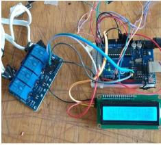
Figure 32 Arduino, relay switch and LCD screen
