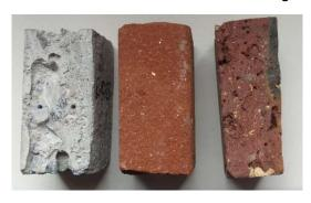
Figure 79 Errors in fabrication: presence of voids, irregular geometry and larger cavities to house thermocouples.
