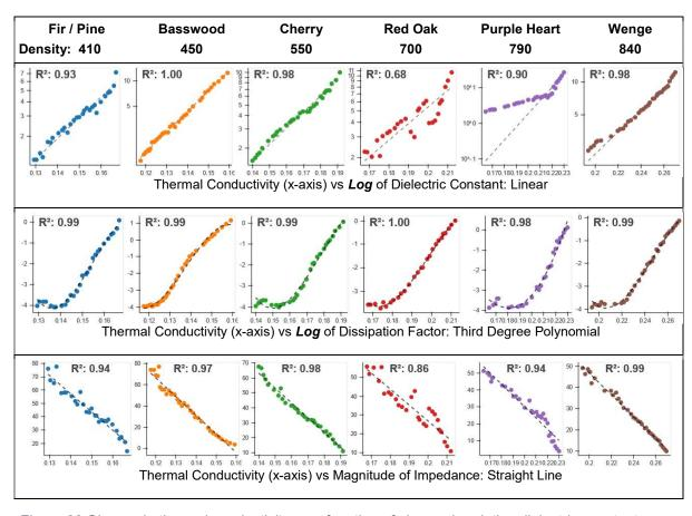
Figure 66 Change in thermal conductivity as a function of change in relative dielectric constant
