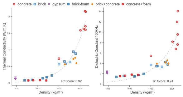
Figure 80 Scatter plot of density and dielectric constant at 100 kHz of the ceramics studied
