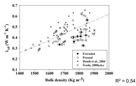
Figure 98 Correlation of bulk density and thermal conductivity for clay bricks as shown by Lassinantti et al [134]
