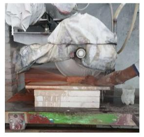
Figure 22 Wet saw (ceramics, cutting)
