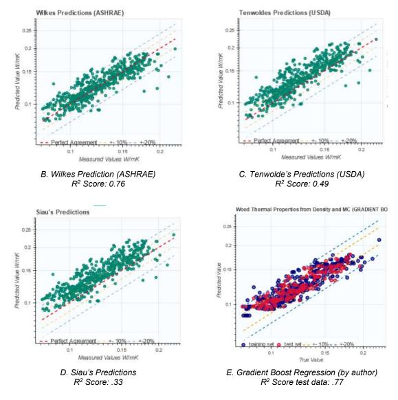
Figure 9 A-E: How equations of various scientists performed on the data collected for wood thermal conductivity.
