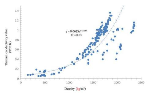
Figure 96 Asadi's [115] data and equation for the correlation of density and thermal conductivity for lightweight concrete
