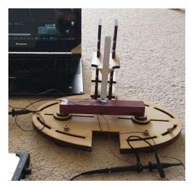
Figure 41 Apparatus for the sound impact method to record sound speed
