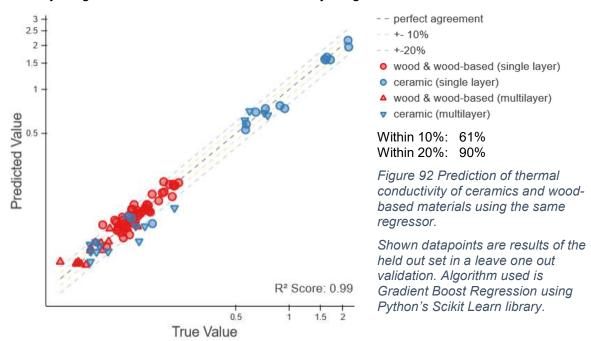
Figure 92 shows the results of leave one out validation where the predicted values of the held-out set are plotted against the true value found by experimentation. The feature space contains three material properties. These are the log of, each of, the dielectric constant, dissipation factor and magnitude of the complex impedance. The algorithm used is a boosting algorithm called gradient boosted decision tree. This specific algorithm was chosen
