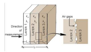
Figure 56 Multilayered material: Layers connected in series. Contact resistance occurs at the interface of two layers because of the roughness of the two surfaces.
