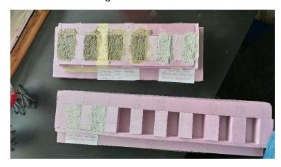
Figure 33 Molds for casting concrete samples
