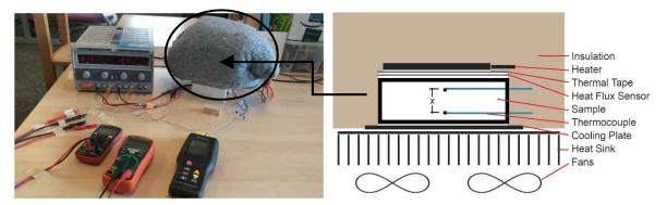
Figure 34: (Left) The instruments used for measuring thermal conductivity. Right: Schematic for the measurement.
