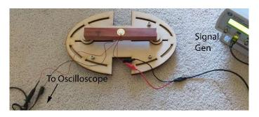
Figure 43 Apparatus for resonance method with signal generator
