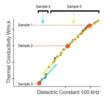
Figure 74 Use of two different blocks to collect data for dielectric properties and thermal conductivity resulted in some errors in the dataset.
