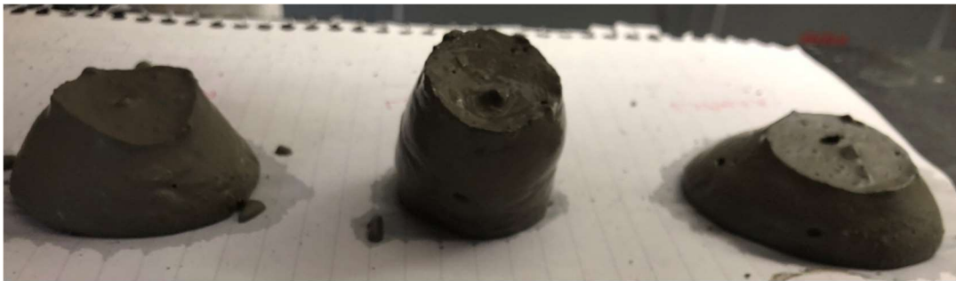
Figure 2.18. On the left is a slump with PMAA graft, the middle is a slump with the 2:1 weight mixture of lignosulfonate and PMAA, respectively, and the slump to the right is LSPMAA.
