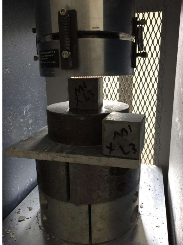
Figure 6.3. Compressive strength samples in the process of being tested.
