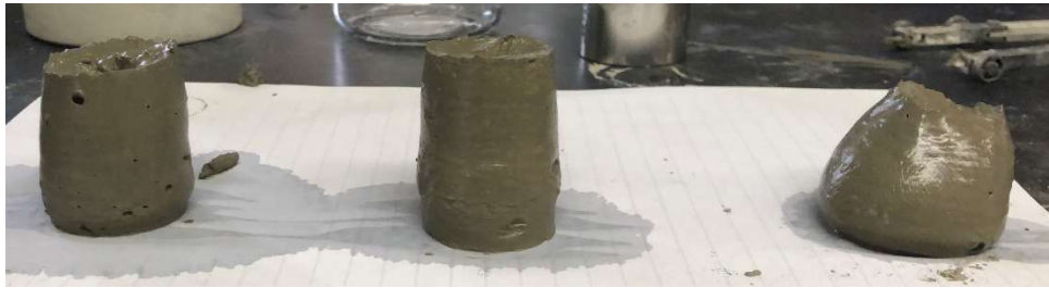
Figure 2.17. On the left is a slump with PEG graft, the middle is a slump with the 2:1 weight mixture of kraft lignin and PEG, respectively, and the slump to the right is KLPEG.
