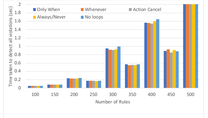
Fig. 4: Performance of SAFETAP: x-axis plots the number of rules in the data-set while y-axis plots the execution time in seconds to detect all violations for different properties.
