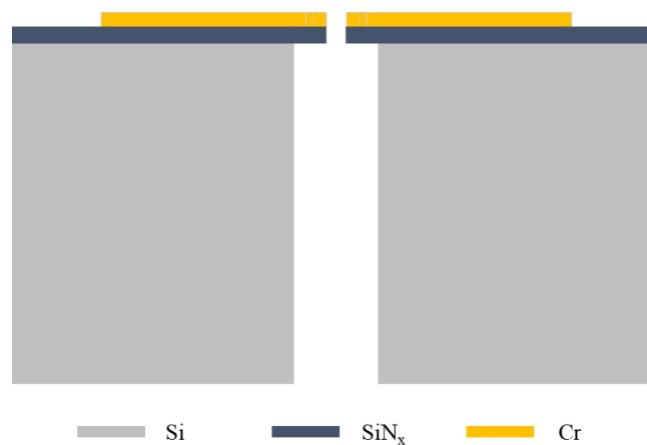
Figure 3-3: Schematic of the substrate design.
