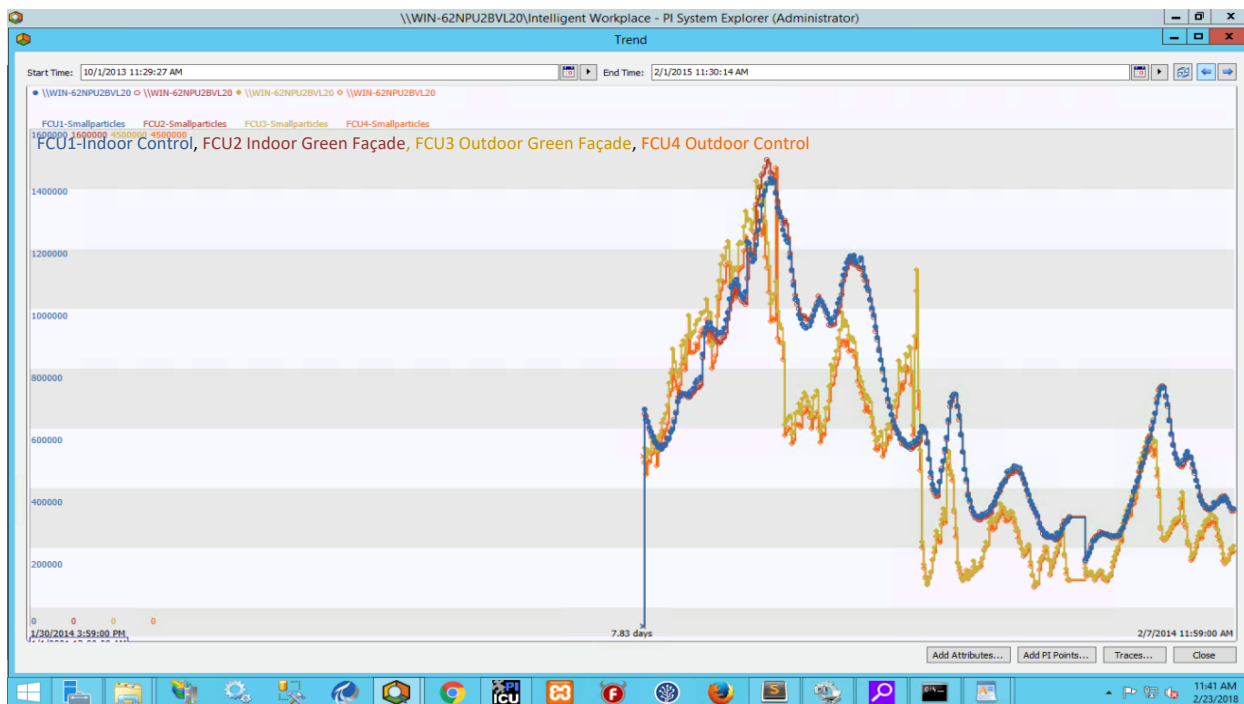
Figure 5.103 1-30-2014 through 2-7-2014, Indoor and outdoor PM2.5 particulate levels are nearly identical for both the green façade and the control façade; this image is an example of the original data representation.
