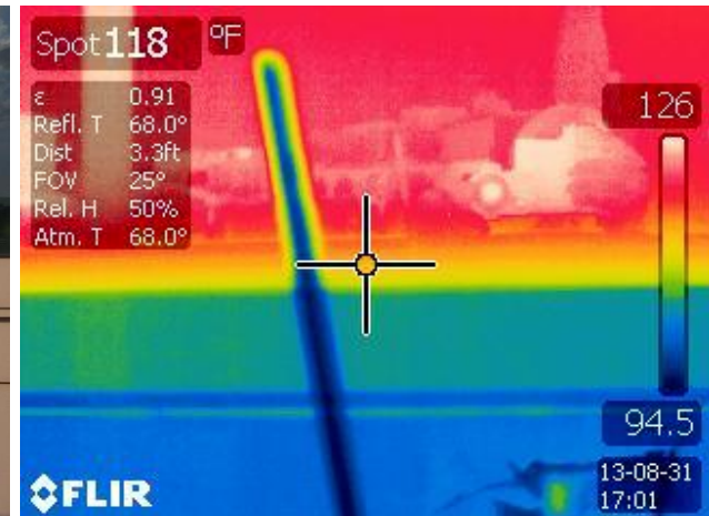
Figure 6.43 Infra-red photo indicating the glazing is approximately 20°F (11.11°C) hotter than the adjacent white aluminum façade panel.
