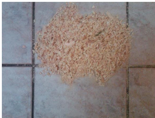
Figure 5.24 Sawdust waste from construction used in fabricated soil mix
