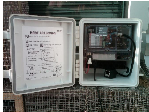
Figure 5.95 HOBO U30 Weather Station connected to sensor cable
