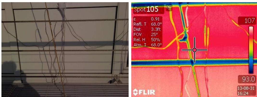
Figure 6.49 Regular photo and thermal image showing 14°F overall temperature range, 2°F spot range at the opaque control façade
