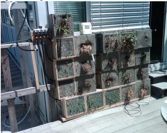
Figure 5.70 The soil moisture sensor connected to the U30
