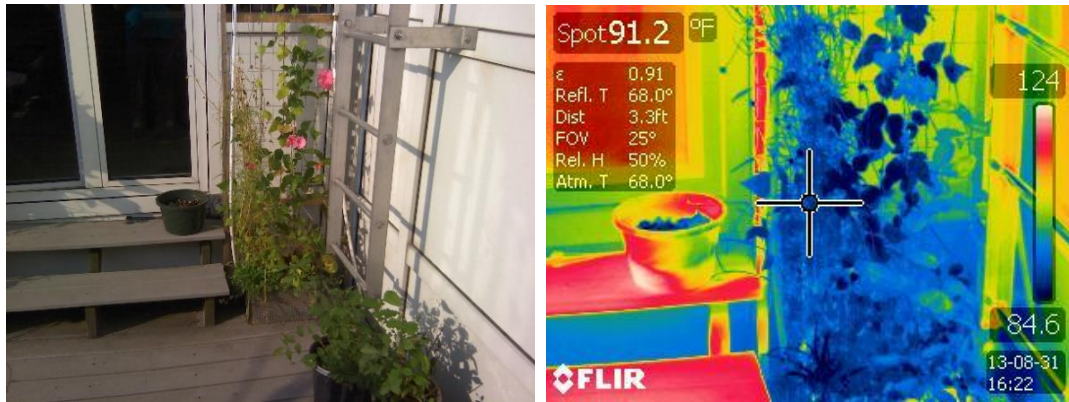
Figure 6.47 Regular photo and thermal image showing 39.4°F overall temperature range, 32.8°F spot range.
