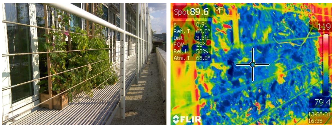
Figure 6.45 Regular photo and thermal image showing 39.6°F overall temperature range, 29.4°F spot range.
