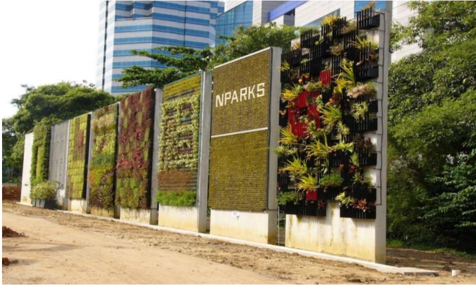
Figure 4.8 Concrete control wall at the far left with eight VGS research systems installed on side-by-side freestanding concrete wall structures (Wong N. H., 2008, p. 27).
