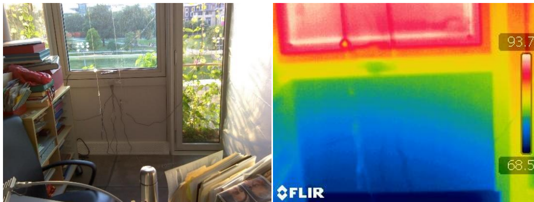
Figure 6.51 Regular photo and thermal image showing 25.2°F overall temperature range, 4.4°F low temperature differential. Living façade is cooler than the control façade.
