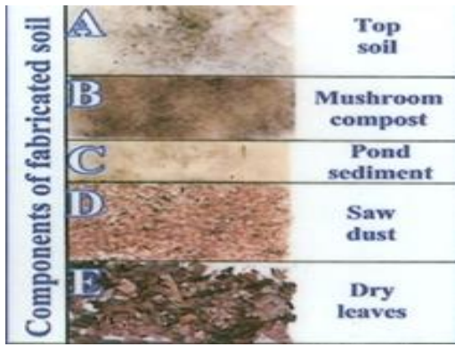
Figure 5.22 The components of fabricated soil (Kefeli, 2013)
