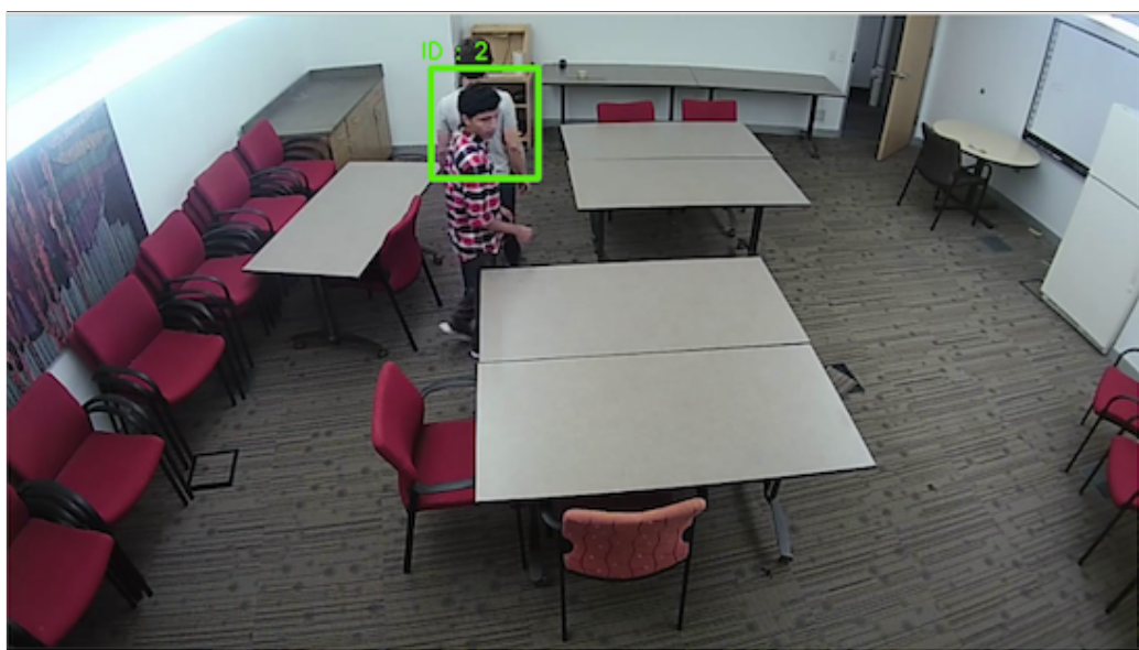
Figure 2: A pedestrian tracker algorithm [1] is applied on test videos. For its performance evaluation, the tracking information (object detection boxes and tracking IDs) on each video is recorded in a Json file.
