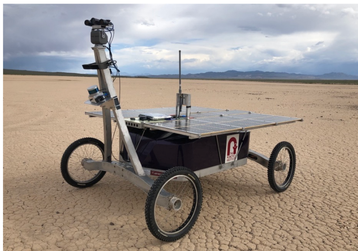
Figure 4.1: Zoë is an autonomous astrobiology rover developed by Carnegie Mellon University. The robot carries various instruments that allow for autonomous science.
