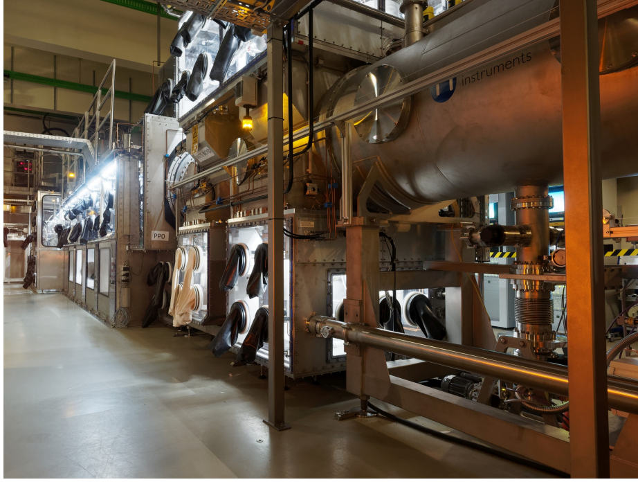
Figure 2.2: KATRIN beamline at the source section. The source chamber is completely obscured by the superconducting magnets and secondary-containment glove boxes. The photograph is taken looking in the downstream direction. Adapted from [49].
