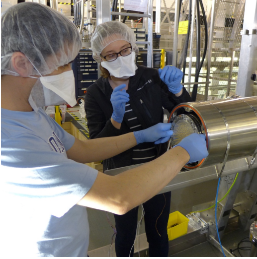
(a) FPD wafer insertion by Florian and Larisa. Courtesy of Florian Fränkle.
