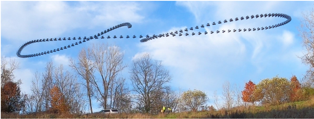
Figure 6.7: Overlay of the 8 m/s 20 meter figure 8 trajectory at Gascola, executed using GPS control.
