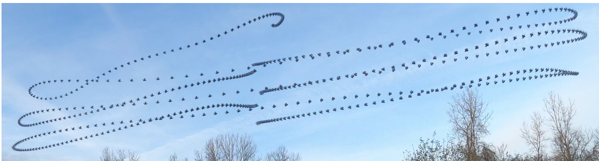
Figure 6.8: Overlay of three high-speed 40 m figure 8 trajectories at Gascola, executed using GPS control. The bottommost trajectory was executed first, with the middle second, and the topmost third. Note the large vertical drift and comparatively lower lateral drift.
