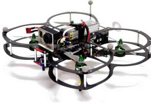
Figure 3.5: The 750g quadrotor used for the hardware experiments. Onboard computation is performed by an Odroid XU4 and the Pixhawk 1 Flight Controller.
