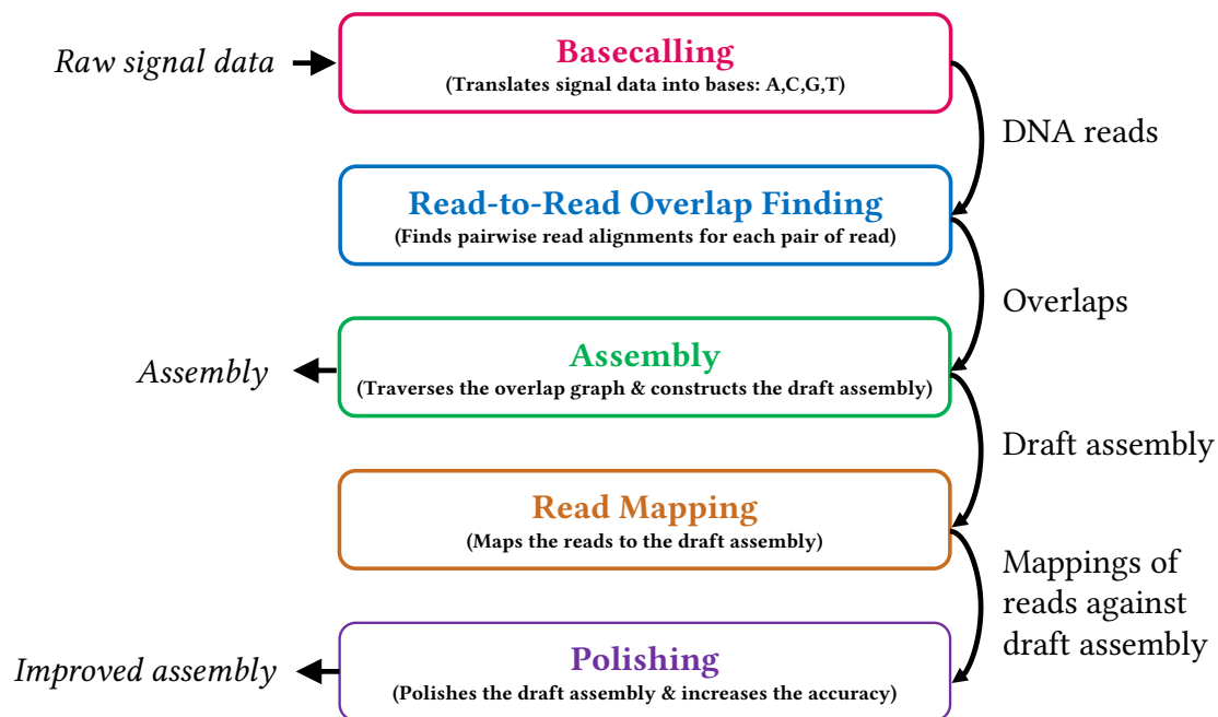
Figure 2-1: Genome assembly pipeline using long reads, with its five steps and the associated tools for each step.
