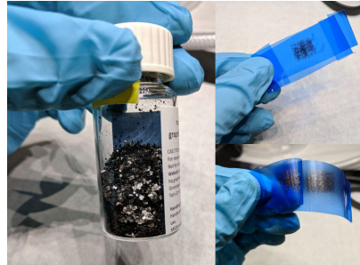
Figure 3.1: Left: bulk graphite flakes. Each flake contains many layers. Right: two pieces of tape sandwiching graphite that is ready to be exfoliated.
