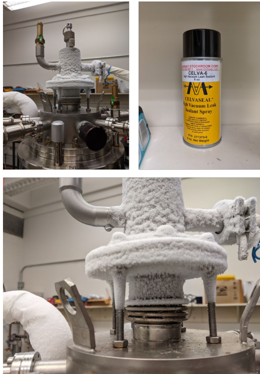
Figure 7.2: a) The steel bellows where the leak occurred. This picture was taken recently after filling the inner cryostat, so a layer of frost is visible over most of the upper portion of the cryostat. A close-up of the bellows is shown in b) , where some rust-colored degradation is visible. Notice the inlet to the LN2 cryostat is just in front of the location of the degradation. c) UHV sealant that was used to close up the leak.
