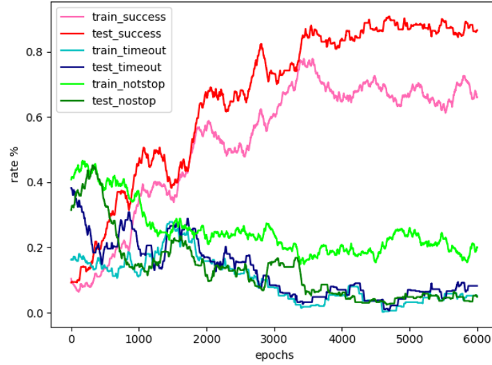
Figure 4.20: Performance rate of Hybrid HRL training process. Results from testing show average performance by testing 500 cases based on the trained network after that training epoch.
