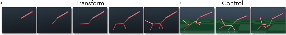
Figure 3.1: Transform2Act learns a transform-and-control policy that first applies transform actions to design an agent and then controls the designed agent to interact with the environment. The giraffe-like agent obtained by Transform2Act can run extremely fast (see video ).
