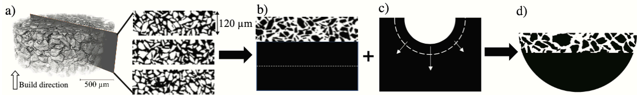
Figure 4.4 Schematics of the Monte Carlo analysis' four-step setup including a) image segmentation from a 2D slice of the \mu\text{XCT} reconstruction of the HDH Ti-6Al-4V powder, overlaying c) a melt pool image on b) a powder bed image, and d) extracting powder bed within the melt pool region.
