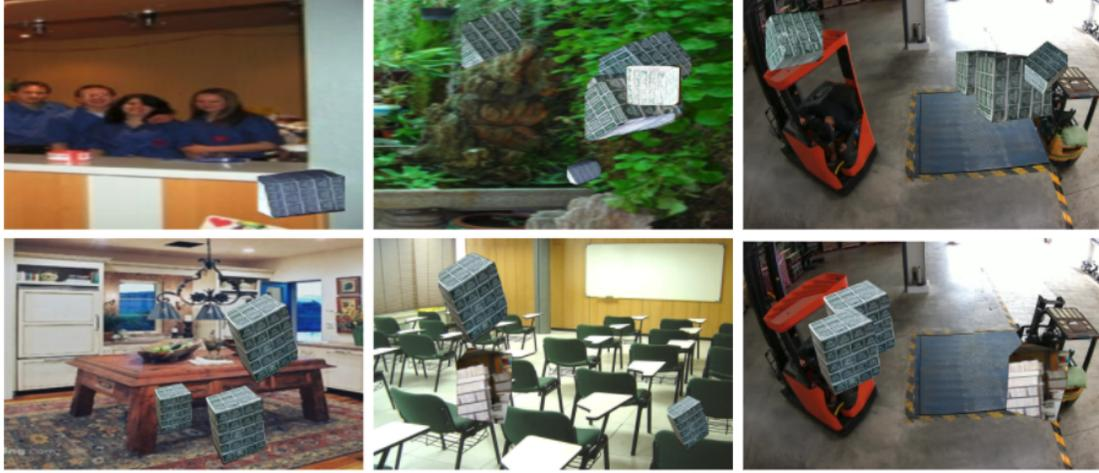
**Figure 4.3:** The top three images show the effect of random dataset generation that lies outside the physical reality of the application. The bottom three images demonstrate the generation process based on PIWIMS linear transformation, color correction and negative sampling.
